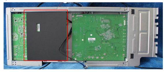
And then remove screws in red, pull out the wire to remove the main board and power board.
