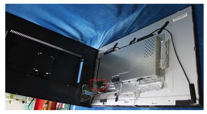
Unscrew the screws and disconnect the connectors to remove the USB board,
