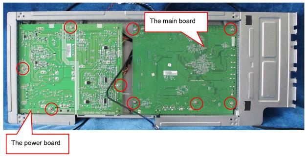
Turn over the power board and main board; remove the cables.
